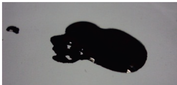
Fig. 1. Physical appearance of Liquefied tropical wood (LTW).
