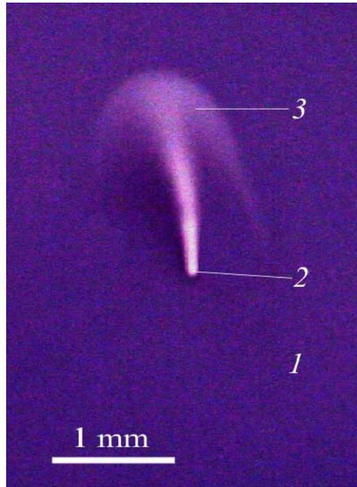
**Fig. 4.** Image of a bleached zone: (1) suspension, (2) zone under irradiation (a focused laser beam was normal to the image plane), (3) bleached suspension upwards by virtue of thermal convection.
