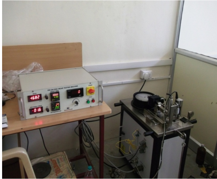
Fig. 3. Photograph of the pin on disc apparatus.
