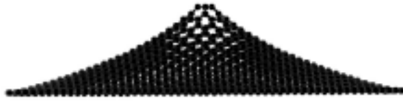
Fig. 1. Deformation of a graphene sheet under a central displacement of 10h .
