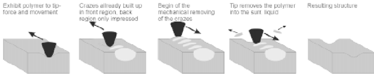
Fig. 5. Model for structuring by usage of polymer crazing. The removed material is left behind in the surrounding liquid.
