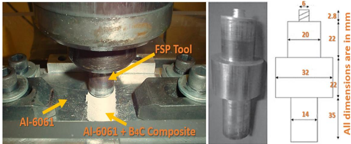
Fig. 2. (a) FSP processing and (b) tool dimensioning
