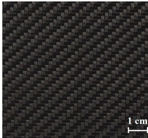
Fig. 1. Optic microscopy image of the surface fragment of the carbon fiber fabric used for the samples making
