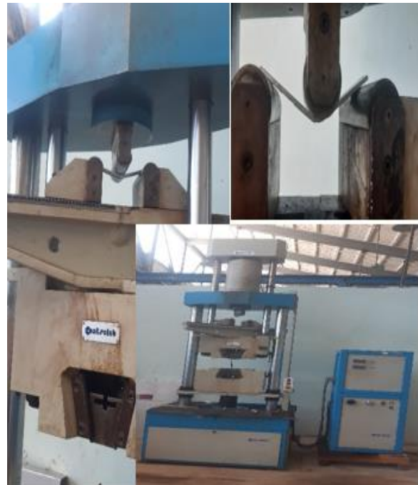
Fig. 5. Testing machine CONTROLAB and specimen for three-point bending test
