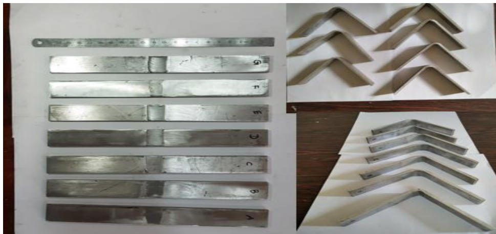
Fig. 8. Three-point bending test
