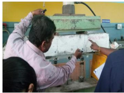
Fig. 18. Marking of cracks
