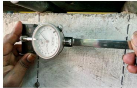
Fig. 17. Strain measurement at 0.42 x_u
