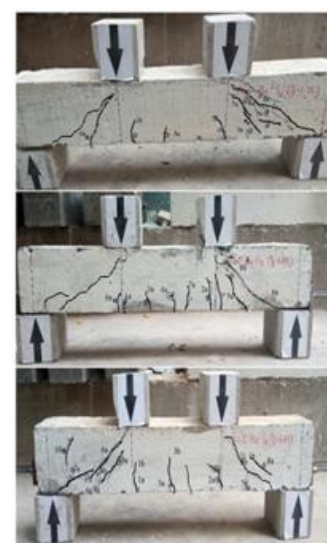
Fig. 23. Pattern of failure of PS-GPC beams
