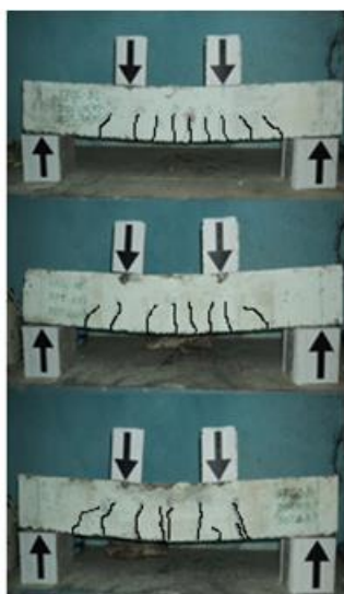
Fig. 21. Pattern of failure of GR-GPC beam
