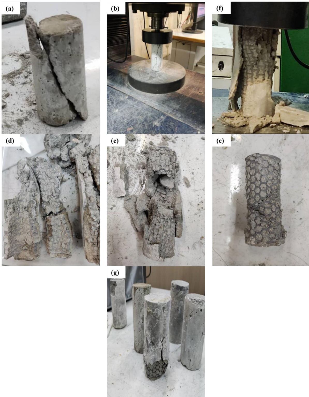
Fig. 13. Failure of STN concrete; (a) control sample; (b) control sample; (c) honeycomb; (d) different of styles of reinforced concrete; (e) RE-85; (f) CA-90; (g) failures of different concrete samples
