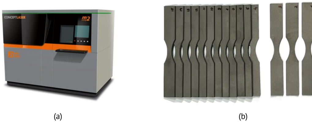
Fig. 6. 3D-printing equipment and prepared Ti-6Al-4V specimens: (a) Concept Laser M2 industrial 3D printer, (b) 3D-printed solid specimens for testing
