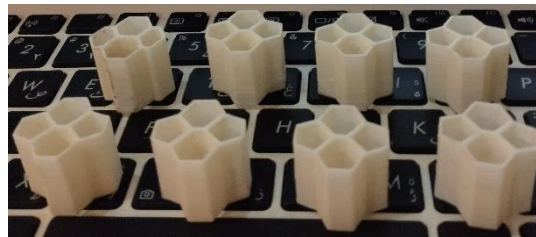
Fig. 3. The scutoid and honeycomb specimens fabricated by 3D printer
