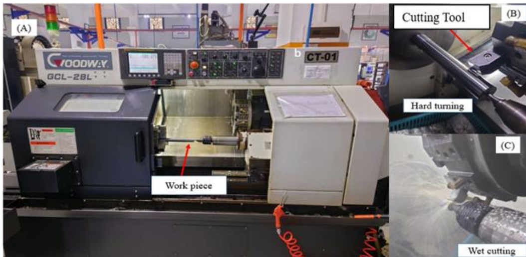
Fig. 2. Experimental setup showing (a) CNC lathe, (b) tool and workpiece, hard turning, (c) wet cutting with coolant
