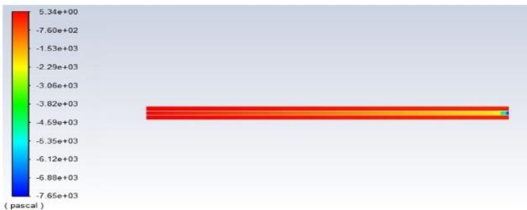
Fig. 10. Pressure contours in an r-z plane along the exchanger for a Reynolds number of 20000 for the water-water exchanger
