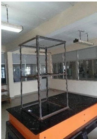
Fig. 1. Two storey steel moment frame
