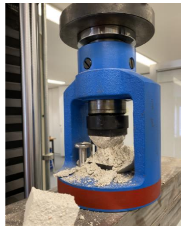
Fig. 2. Specimen condition after reaching the breaking load during the bending test
