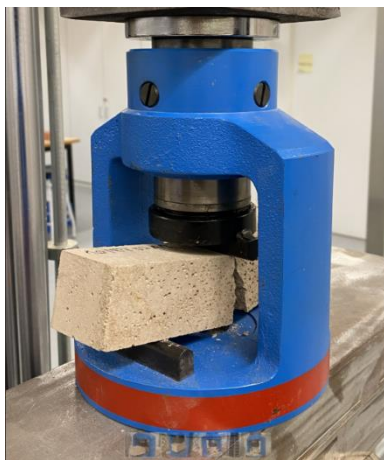
Fig. 1. Three-point bending test on prismatic mortar specimens
